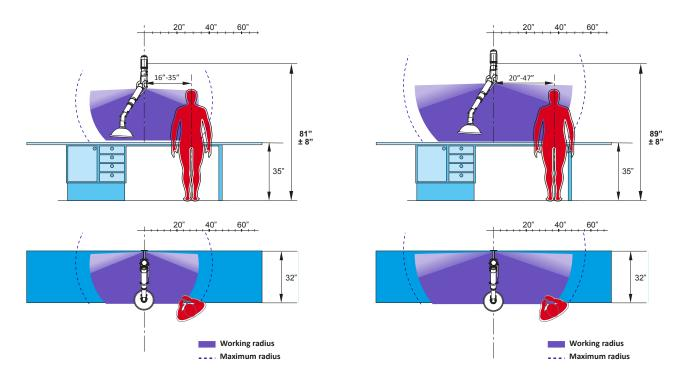
To optimize the usability of the extractor, the above mentioned mounting heights, and sideways displacements from the workplace, are recommended.
