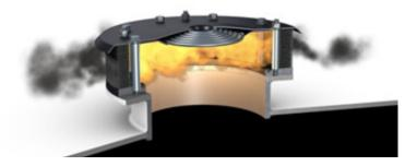
arrester is used to dissipate the energy of the expelled combustion flames into its material. By reducing the gas temperature to a safe level, flameless venting can be used in areas where it would be impossible to safely use an explosion vent only.
