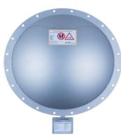
Filter installations with pneumatic cleaning systems and a very high vacuum operation require an explosion vent that withstands vacuum and positive pressure cycling for a long time. For such requirements the GE is the best choice. Its domed design enables negative pressure resistance without the need for an extra vacuum support. The GE type vents feature pressure peak damping as well as integrated flange gaskets.
