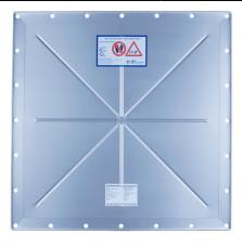
The KER style vent is perfect for standard applications in powder handling and storage. The KER is suitable for plant equipment with static over/under pressure conditions up to 50% of the rated rupture pressure. A unique feature with the KER is that edge reinforcement in its design allows the KER to be mounted without an outlet flange thus reducing installation costs. Cross rib and folded edges are standard KER design features. Each vent comes with an integrated flange gasket.
