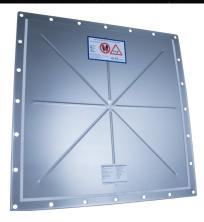
If the negative pressure is not greater than 60% of the rated rupture pressure, installation of a domed vent has no extra benefit. For this application the KE is an alternative to the domed GE. The KE provides long durability and aerodynamic advantages compared to the domed type, for example in cyclones. Pressure spike dampening, integrated flange gaskets, cross rib and folded edges are standard KE design features.
