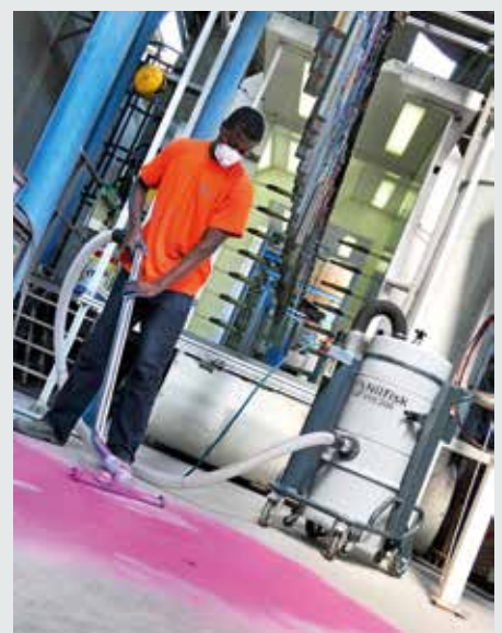
Recovery of epoxy powder from all surfaces
