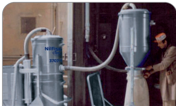
Vacuuming large volumes of grain and discharging directly into bags
