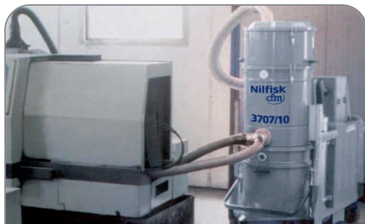
Continuous suction at the source of the debris
