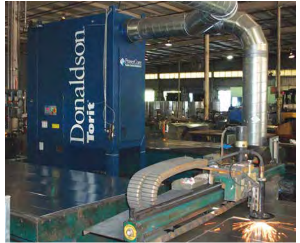
TG on Plasma Cutting 3,400 cfm (5,775 m 3 /h)
