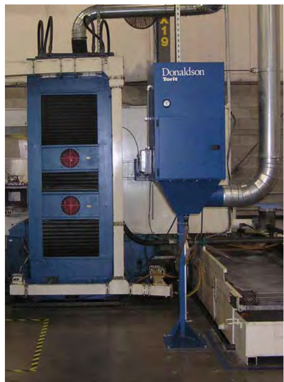
WSO - Horizontal Grinder 850 cfm (1,444 m 3 /h)
