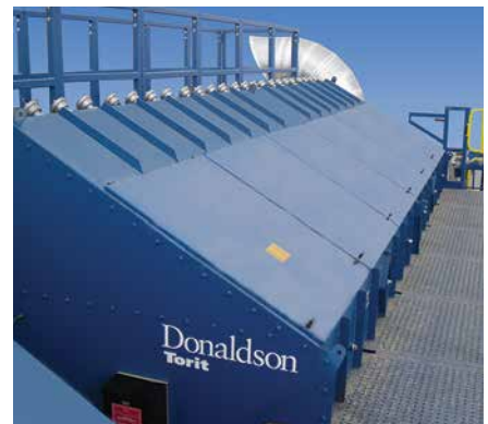
CPC - Grain Tripper Conveyor 18,700 cfm (31,765 m 3 /h)
