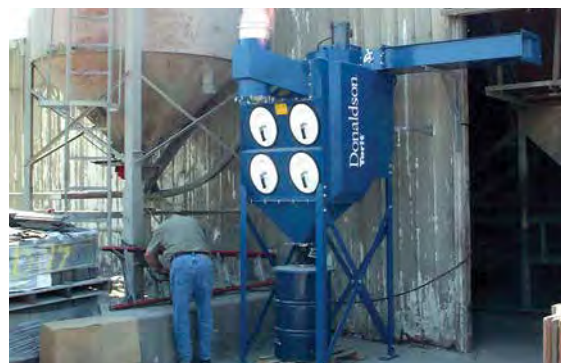
DFO - Concrete Roof Manufacturer 3,000 cfm (5,096 m³/h)
