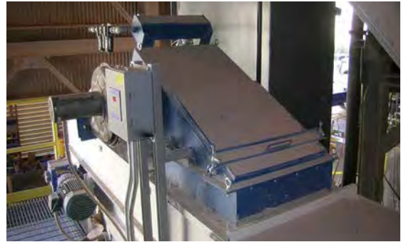
CPV - Weigh Belt Feeder 800 cfm (1,359 m³/h)
