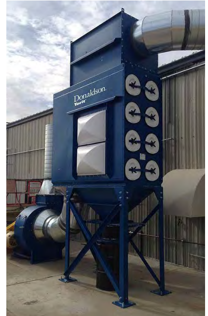
DFO on Plastics Routing 16,000 cfm (27,184 m 3 /h)
