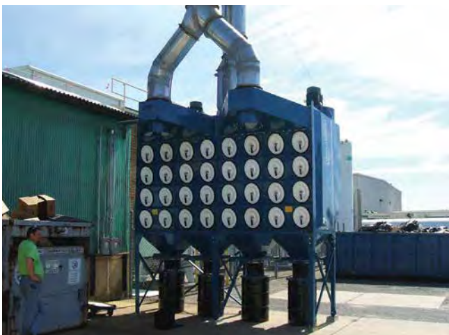
DFO on Thermal Spray 8,500 cfm (14,439 m 3 /h)
