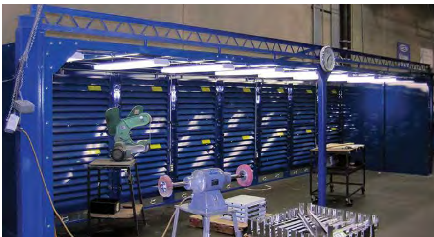
DWS on Custom Hand Grinding 38,500 cfm (65,398 m³/h)
