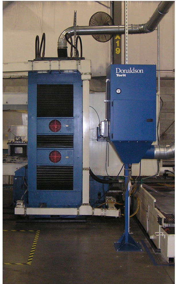
WSO - Horizontal Grinder 850 cfm (1,444 m 3 /h)
