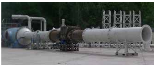
Flap valve test with INERIS notified body
